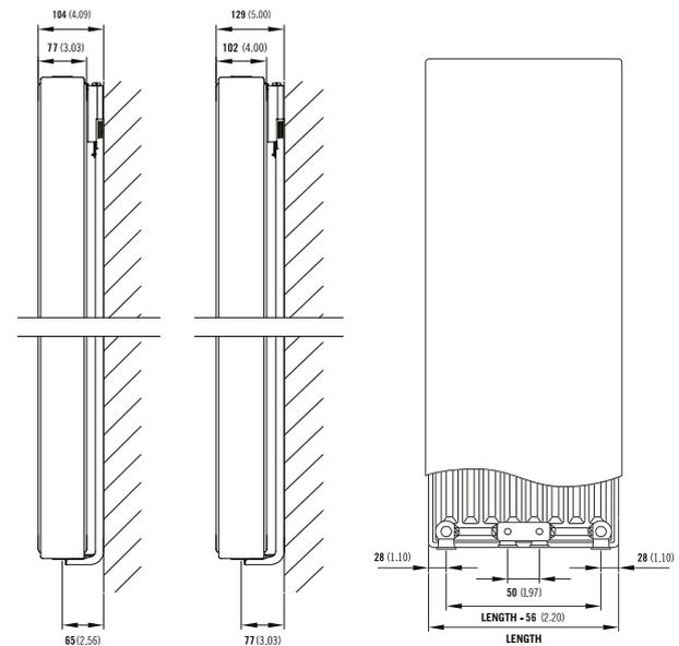
**Connections** Each radiator comes with 1/2" inlet connections as standard.
