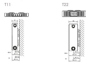
**Bracket Position** A = Closest to wall, B = Furthest from wall, (R) = Recommended unting position.
