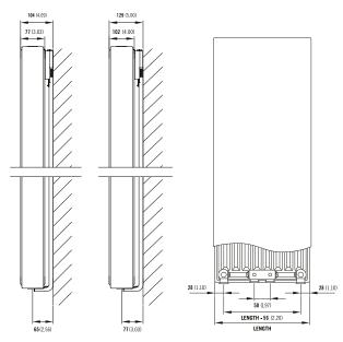
Connections Each radiator comes with  $1/2^{\prime\prime}$  inlet connections as standard.
