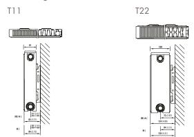
**Bracket Position** A = Closest to wall, B = Furthest from wall, (R) = Recommended unting position.
